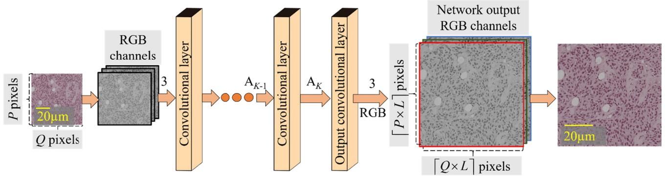
**Fig. S5.** Detailed schematics of the deep neural network high-resolution image inference (i.e., the testing phase).
