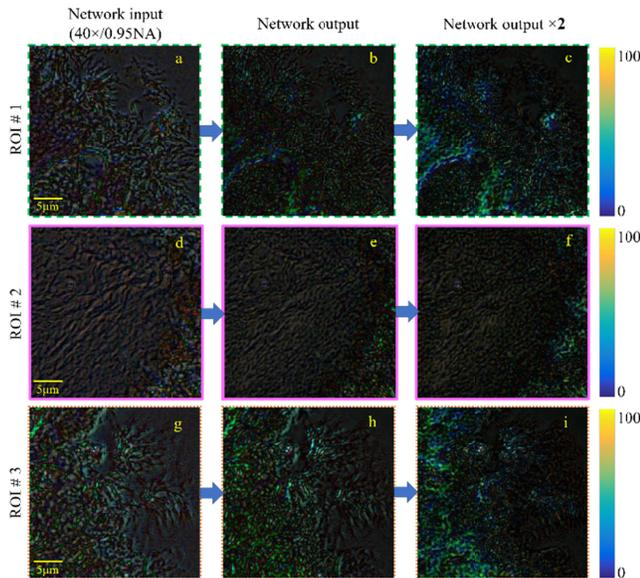
**Fig S7.** The percentage of the pixel-level differences for the network input or output images calculated with respect to the gold standard images captured using a 100x/1.4NA objective lens. ROIs correspond to the Masson's trichrome stained lung tissue shown in Fig. 2 of the main text. The colorbar spans 0-100%.
