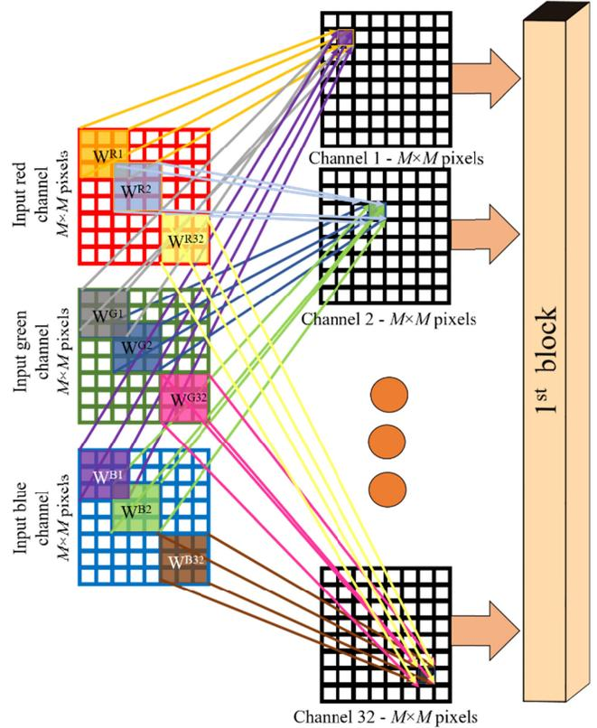
**Fig. S2.** Detailed schematics of the input layer of the deep neural network.
