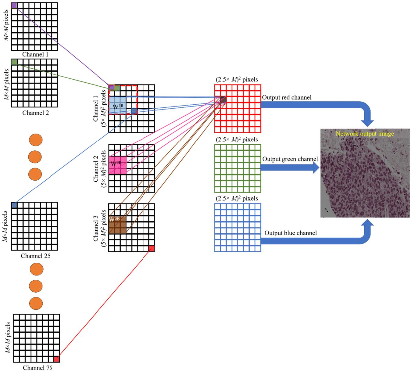
**Fig S3.** Detailed schematics of the output layer of the deep neural network for  $L=2.5$ .
