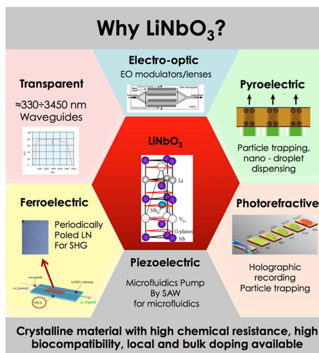
Figure 3. The main properties of lithium niobate (LiNbO 3 ).
